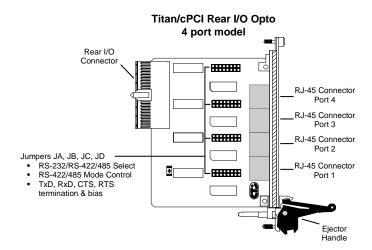
Figure 5: Titan/cPCI Rear I/O Opto two and four port adapters.
